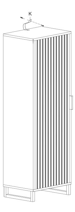
Fitting K should be used to secure your ST CALX LOCKER to the wall. Screws and fittings for wall are not supplied as different wall constructions require fittings that are suitable for your wall type. If you are unsure for the correct type of fitting for your wall, please contact your local specialised hardware store for information on suitable fitting.
