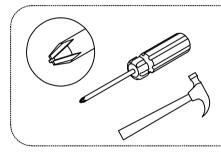
You will need a cross head screwdriver and a hammer to assemble this product. An electric drill may cause damage and is not recommended.
