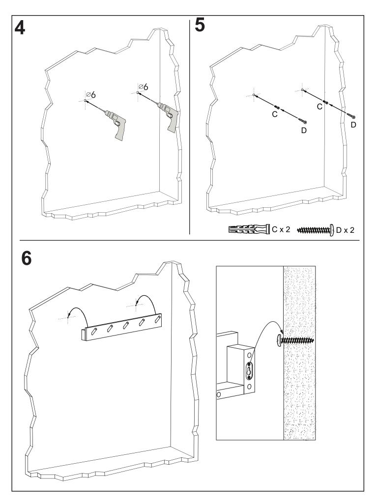
Fittings to attach this product to the wall are supplied. But different wall constructions require fittings that are suitable for your wall type. If you are unsure for the correct type of fitting for your wall, please contact your local specialised hardware store for information on suitable fitting.
