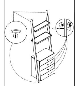
To ensure that the unit remains stable, either use fixing hole to fix it to the wall or apply the Anti-slip pads to the ends of the rails.
