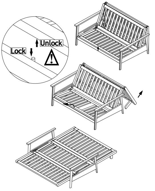
**CONVERTING YOUR SOFA INTO A BED** Slide the back and seat deck in the direction of the arrows. After opening ensure that the frame is locked into position.
