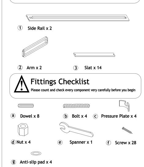
Cross head Screwdriver also required for assembly
