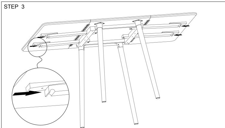
To close table, hold tabletop whilst sliding support into centre. To open, do the reverse.
