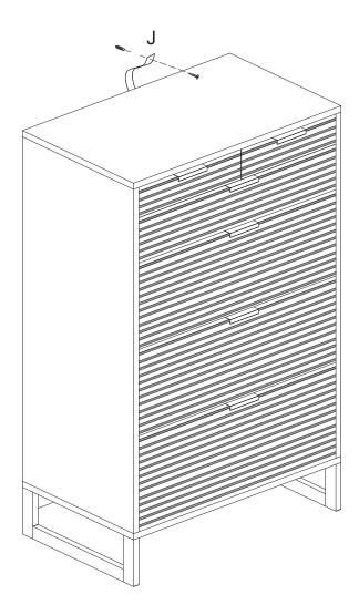
Fitting J should be used to secure your ST COD CALX to the wall. Screws and fittings for wall are not supplied as different wall constructions require fittings that are suitable for your wall type. If you are unsure for the correct type of fitting for your wall, please contact your local specialised hardware store for information on suitable fitting.
