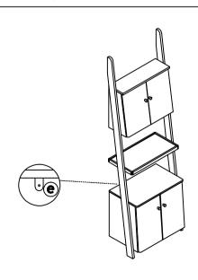
Fittings to secure your Cabinet to the wall are not supplied. But different wall constructions require fittings that are suitable for your wall type. If you are unsure of the correct type of fitting for your wall, please contact your local specialised hardware store for information on suitable fitting. For safety reasons, we advise you to fix this item to the wall if young children or boisterous dogs are liable to bang into it. Never allow children to climb on furniture.
