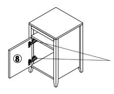
Fix these screws first when attaching doors to cabinet unit.
