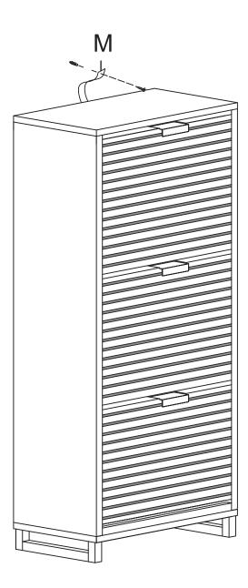
Fitting M should be used to secure your ST CALX SHOE CAB to the wall. Screws and fittings for wall are not supplied as different wall constructions require fittings that are suitable for your wall type. If you are unsure for the correct type of fitting for your wall, please contact your local specialised hardware store for information on suitable fitting.
