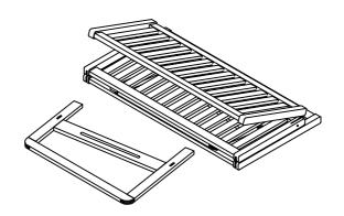
Then lift up the two sections of wooden deck to safely remove the second wooden arm.
