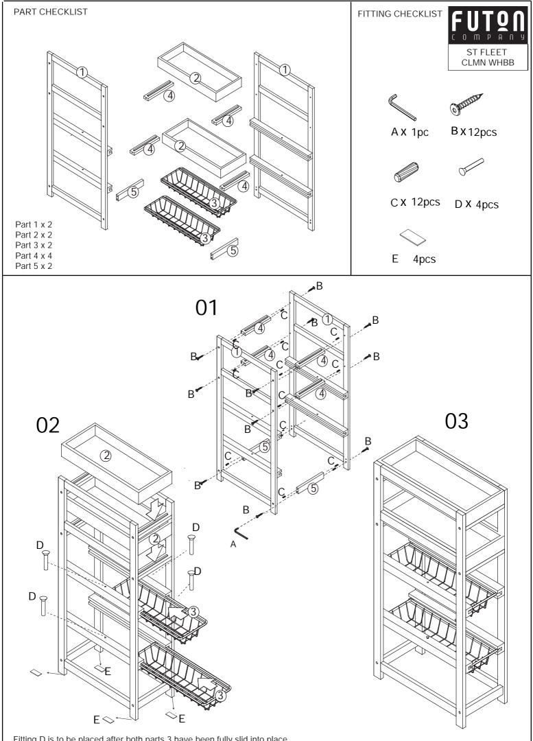
Fitting D is to be placed after both parts 3 have been fully slid into place
