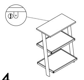
Fittings to secure your shelf to the wall are not supplied. But different wall constructions require fittings that are suitable for your wall type. If you are unsure of the correct type of fitting for your wall, please contact your local specialised hardware store for information on suitable fitting.
